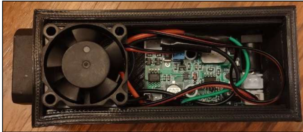
Figure 5: White laser with cooling fan
