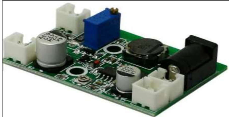
Figure 6: Laser control board
